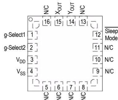
**Figure 1. Pin Connections**
