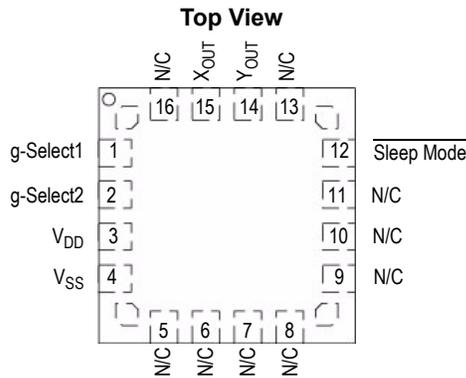
Figure 4. Pinout Description
